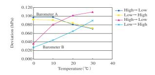
F 5. Characteristics of hysteresis of the tested barometers
